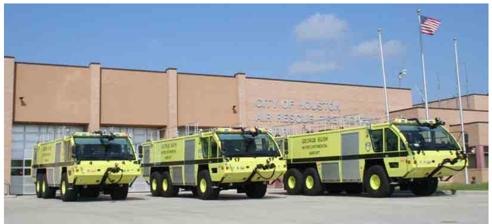
(RIGHT) The City of Houston (Texas, USA) recently took delivery of five (5) Rosenbauer Panthers with the (HPCS) suspension system. Three (3) 3,000 gallon 6x6 units, one (1) 1,500 gallon 4x4 and one (1) 3,000 gallon 6x6 with HRET. The 3,000 gallon 6x6 Panthers will be stationed at George Bush Intercontinental Airport, with the remaining 4x4 and 6x6 HRET stationed at William P. Hobby Airport. (Photo: Rosenbauer)
