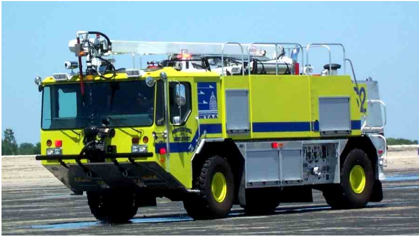
(LEFT) Metropolitan Topeka (Kansas) Airport has taken delivery of a 2006 Emergency One TITAN HPR 4X4 crash truck. The vehicle carries 1500 gallons of water, 105 gallons of foam and is equipped with a Hale 1500 gpm pump. It is powered by a Detroit Diesel Series 60 665HP engine and a Twin Disc transmission.
