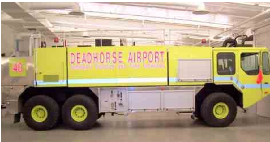
LEFT: Emergency One (E-One) has delivered a TITAN HPR 6X6 vehicle to Deadhorse Airport in Alaska, and a similar unit to Cordova Airport, also in Alaska. The vehicles carry 3000 gallons of water, 400 gallons of foam and 50 pounds of dry chemical.
