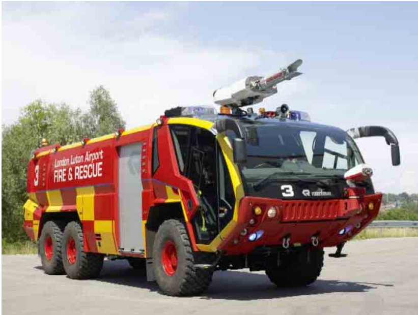
LEFT: London Luton Airport Fire & Rescue Service (UK) has taken delivery of new Rosenbauer PANTHER CA-5 6X6 airport crash truck. The truck is based on a Model RBM 36.705 6X6 chassis and is powered by a Caterpillar C-18 six cylinder diesel engine with a Twin-Disc transmission. The firefighting package includes a Rosenbauer R600 pump rated at 7,000 lpm at 15 Bar, and Rosenbauer FOAMATIC RVMA 500 foam pump. The vehicle carries 12,500 liters of water and 1,500 liters of foam. It carries an ancillary dry chemical system of 225 kg. It is designed to carry a crew of a driver and 3 firefighters. The unusual paint scheme is very distinctive.
