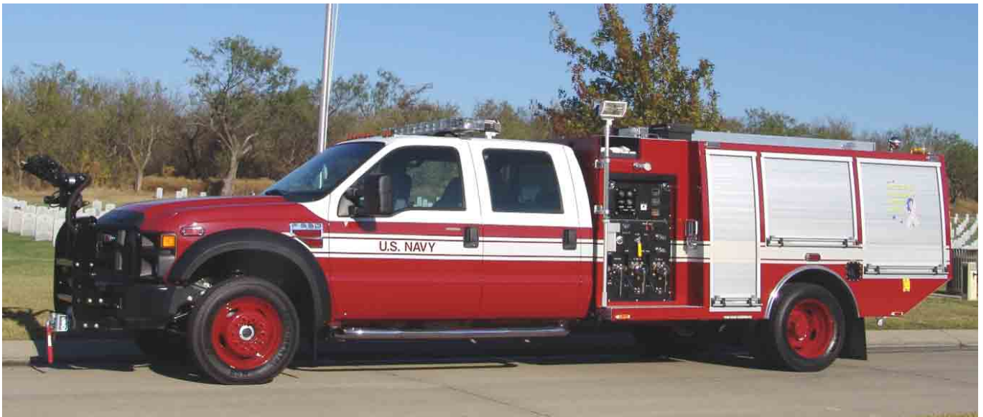
MIDDLE: Crash Rescue Equipment Service, Inc. recently delivered six (6) Renegade™ CAV-2400 Aircraft Fire-fighting Vehicles to the U.S. Navy which feature a custom PolyBilt Body as well as a Darley 2 ½ AGE 250 gpm Deutz pump. The chassis is a Ford F-550 4X4 model with a diesel engine and automatic transmission. The fire package consists of a 400 gallon water tank with a 50 gallon foam reservoir which are integral with the body and 200 lbs of dry chemical. The truck features a remote controlled bumper turret, Hydro-Chem technology for maximum firefighting capabilities plus a stored air compressed air foam system.
